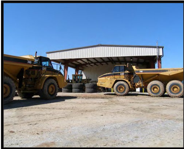
Off-Road Trucks Used To Hall Cover
